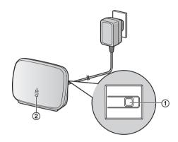
The indicator lights when the registration is completed. (Depending on the signal status, the indicator may not light in green. In this case, see the repeater's Getting Started.)
