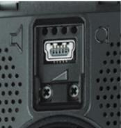
Mini-USB connection and loudspeaker/ microphone volume adjustment
