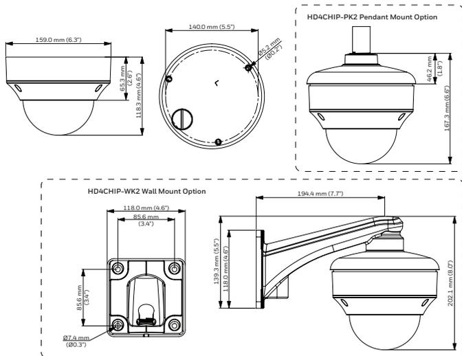
\* Dimensions drawing shows mounting plate. Mounting plate is compatible with a 4S electrical box.
